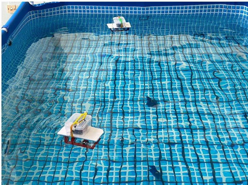
In both the land and sea-based transportation systems, they learnt to use the radio built into the micro:bit to control their vehicles remotely.
